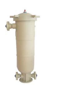
Plastic Bag Housing is made of 100% pure German made Polypropylene resin, by integrated one-piece injection molding technologies, featuring excellent resistance to pressure, corrosion and ultraviolet light attack. It is designed to use industrial standard Size two filter bags (Ø 7" X 32"long ); Filter Housing has broad applications, and is ideal for high flow, corrosive and outdoor applications.
