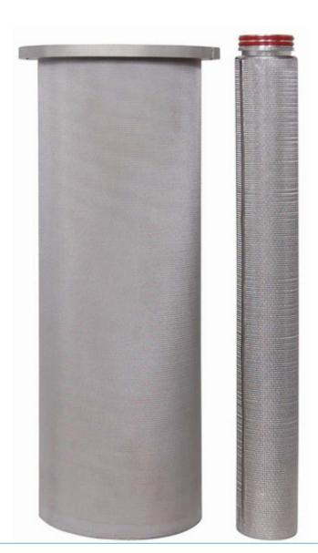
Sintered multilayer wire mesh bags are designed for high temperature Application of Industries. It can be used for high temperature up to 480°C. It has one standard combination of 5 Layers sintered wire mesh made from stainless steel which is brought together through vacuum sinter, compression and rolling and made into a kind of porous material.
